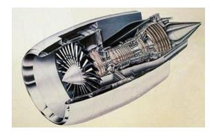
GE90 Turbofan Engine is the largest and most powerful engine in the world with versions. The fan diameter is 12 ft (4 meters) developing in excess of 100,000 pounds of thrust.
